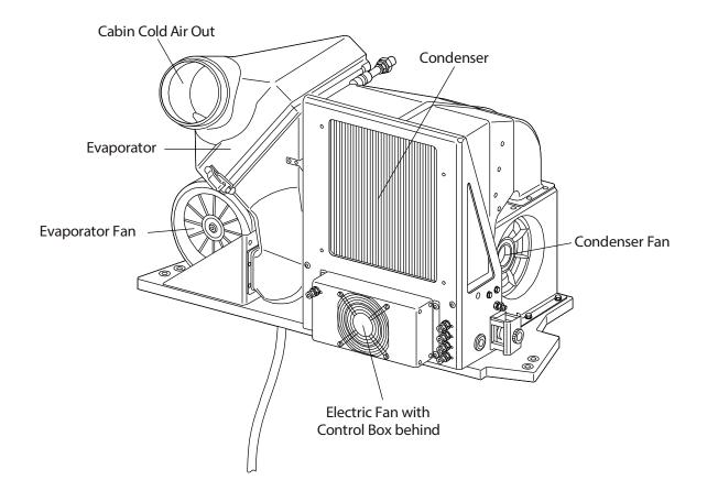
Figure 202 : Central Unit - Front and LH Side (if OÄM 40-316/i or later installed)
