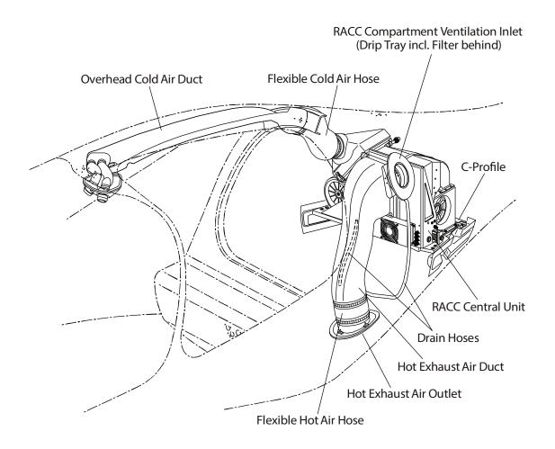
Figure 201 : RACC Central Unit Installation (if OÄM 40-316/i or later installed)
