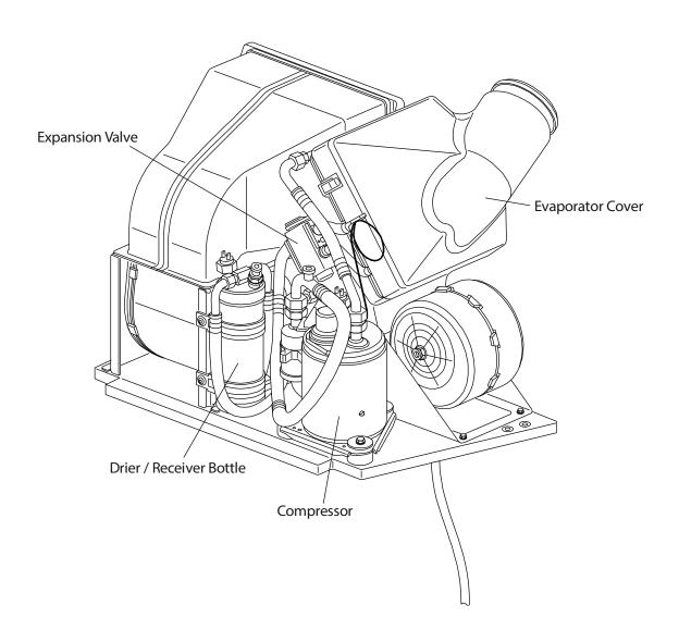
Figure 203 : Central Unit - Back and RH Side (if OÄM 40-316/i or later installed)
